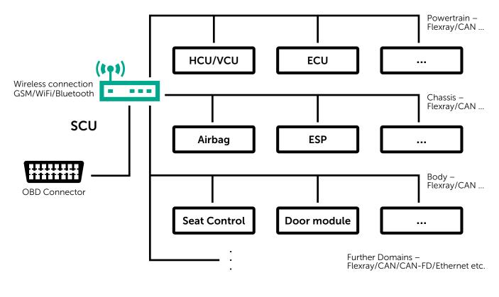
The SCU is a communication gateway control unit, connected to several subnets and/or gateway controllers to those subnets within the car network. Thus, the SCU is a single gateway to external communications, whereas internal devices can communicate within a domain or even between domains without using SCU services.
