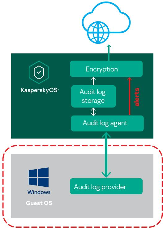
With KSH it's possible to prevent audit log spoofing in a guest OS. A trusted channel between KSH and the guest OS makes it possible to deliver the audit log that's securely stored in KSH (there's a range of options for protecting the log – from storing it as a file on the KSH side to a blockchain-based approach that guarantees spoofing protection even if a device is physically accessed).
