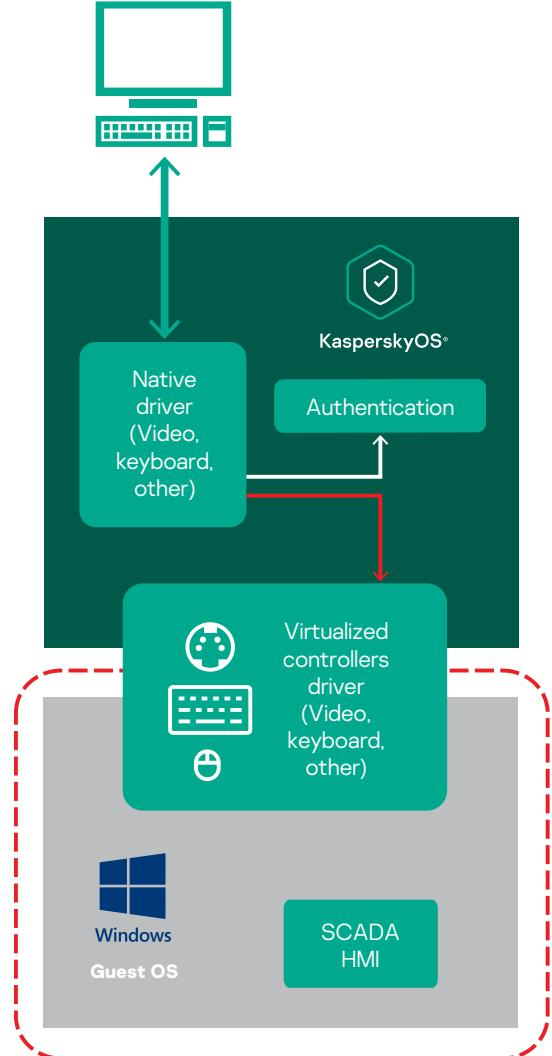
Because guest OSs are complex systems and can include many vulnerabilities and problems, we can't trust their native authentication mechanisms. KSH operates in a trusted environment, so can provide additional independent and reliable authentication on the KasperskyOS level.
